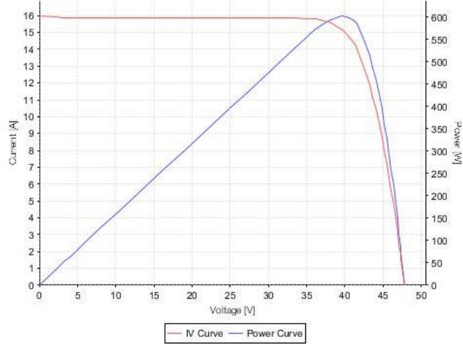
Fig. 5 IV curve of module No.1 Serial number: ASA29200300201
